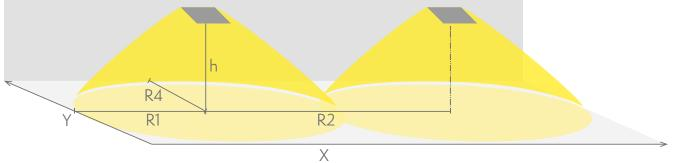
R1 distance from wall (X axis) R2 installation distance between lights (X axis) R4 distance from wall (Y axis) TWS9292WMC
