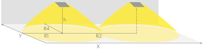
R1 distance from wall (X axis) R2 installation distance between lights (X axis) R4 distance from wall (Y axis) TWS9992WA
