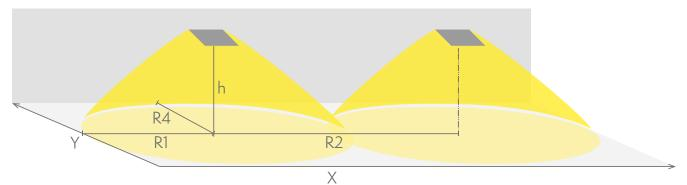
R1 distance from wall (X axis) R2 installation distance between lights (X axis) R4 distance from wall (Y axis) TWSA192WM
