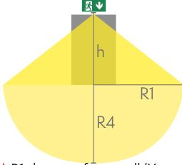
R1 distance from wall (X axis) R4 distance from wall (Y axis) TWT3071WE
