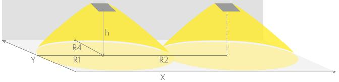
R1 distance from wall (X axis) R2 installation distance between lights (X axis) R4 distance from wall (Y axis) TWT9253WM
