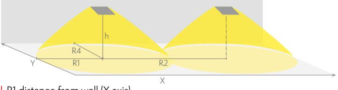
R1 distance from wall (X axis) R2 installation distance between lights (X axis) R4 distance from wall (Y axis) TWTB152WA
