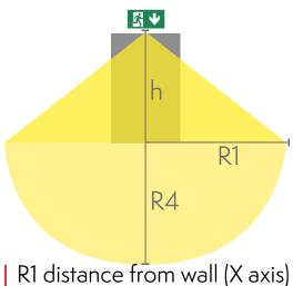
R1 distance from wall (X axis) R4 distance from wall (Y axis) Y8051W105
