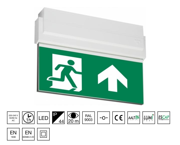
Self-contained ESCAP Emergency Exit Light with 1 h Super Capacitor and Wireless Central Monitoring, with 2-sided pictogram, arrow up, 20 m viewing distance (Invidually packed TWS8092WA)
