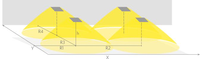
R1 distance from wall (X axis) R2 installation distance between lights (X axis) R3 installation distance between lights (Y axis) R4 distance from wall (Y axis) Y9292WA
