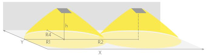
R1 distance from wall (X axis) R2 installation distance between lights (X axis) R4 distance from wall (Y axis) Y9292WA
