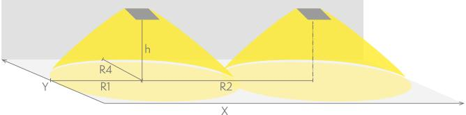
R1 distance from wall (X axis) R2 installation distance between lights (X axis) R4 distance from wall (Y axis) TWS4292WA
