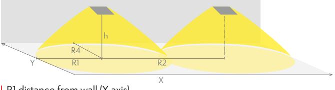
R1 distance from wall (X axis) R2 installation distance between lights (X axis) R4 distance from wall (Y axis) TWTB171W
