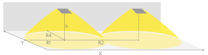
R1 distance from wall (X axis) R2 installation distance between lights (X axis) R4 distance from wall (Y axis) TWTC252WA
