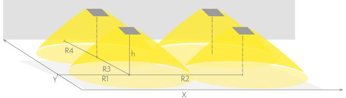
R1 distance from wall (X axis) R2 installation distance between lights (X axis) R3 installation distance between lights (Y axis) R4 distance from wall (Y axis)
