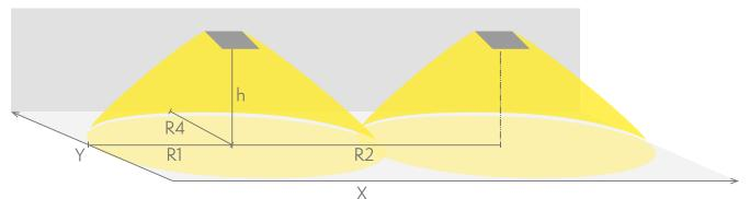
R1 distance from wall (X axis) R2 installation distance between lights (X axis) R4 distance from wall (Y axis) TWTC271W
