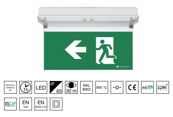
Self-contained Escap emergency exit light with 1 h super capacitor and wireless central monitoring, with 1-sided pictogram, arrow left, 30 m viewing distance (Invidually packed TWS3192WA)
