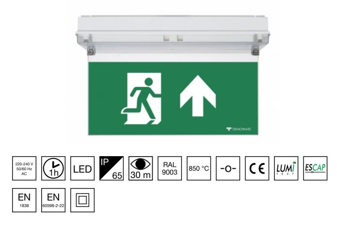
Self-contained Escap emergency exit light with 1 h super capacitor and Lumi Test self-testing with 2-sided pictogram, arrow up, 30 m viewing distance (Invidually packed TWS3192WM)
