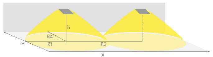
R1 distance from wall (X axis) R2 installation distance between lights (X axis) R4 distance from wall (Y axis) Y4352WA
