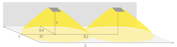
R1 distance from wall (X axis) R2 installation distance between lights (X axis) R4 distance from wall (Y axis) Y8852WA
