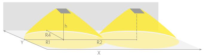
R1 distance from wall (X axis) R2 installation distance between lights (X axis) R4 distance from wall (Y axis) Y9253WA
