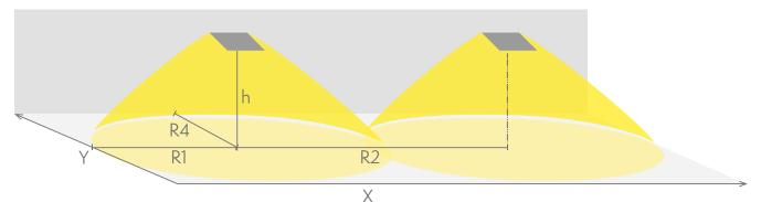
R1 distance from wall (X axis) R2 installation distance between lights (X axis) R4 distance from wall (Y axis) Y9952WM
