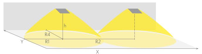
R1 distance from wall (X axis) R2 installation distance between lights (X axis) R4 distance from wall (Y axis) Y9992WM
